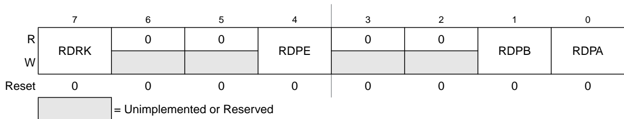
Figure 18-15. Reduced Drive Register (RDRIV)
